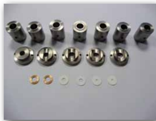
Adaptors and reducer rings allows to analyze even small samples and thin wires
